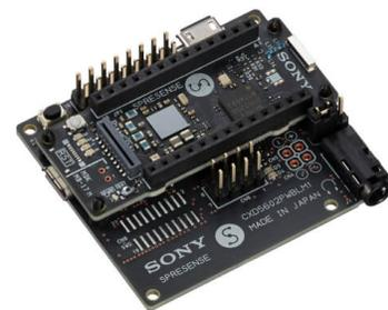
**Sony's SPRESENSE microcontroller with LTE Connectivity from Soracom**
